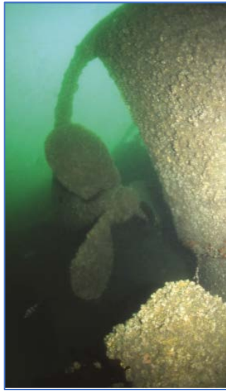
Port Propeller (cone missing) & aft hydroplane. Image Martin Davies
